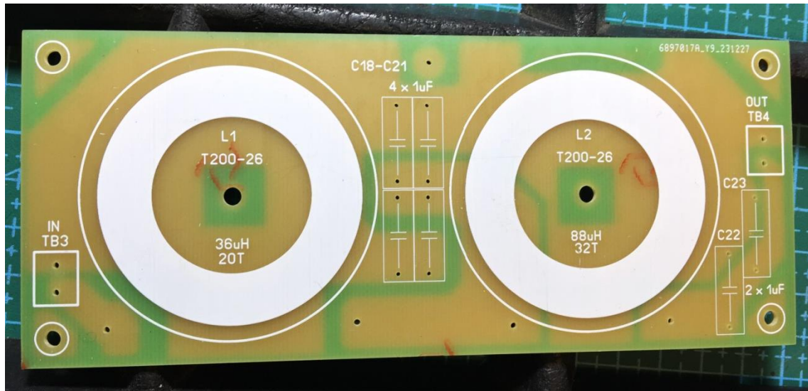
Figure 10 LPF PCB layout.
